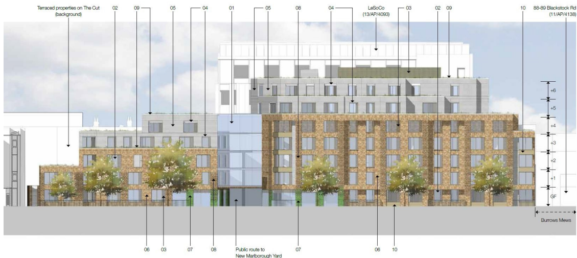
Figure 6: The proposed Ufford Street elevation. The glazed 'bridge' links Block A (on the left) to Block B (on the right)
